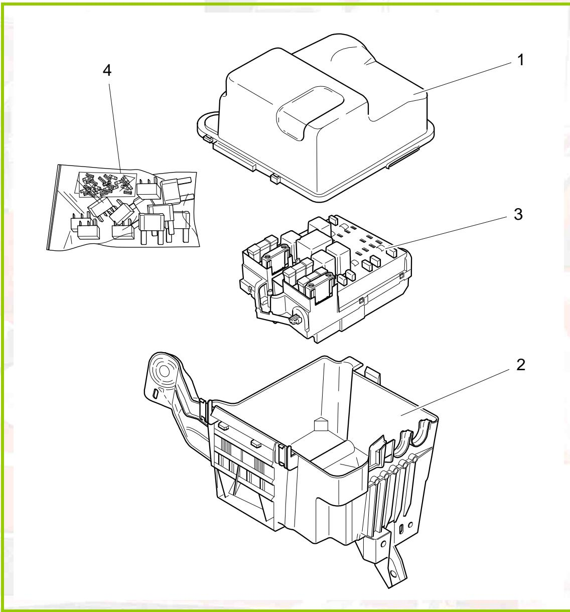
Fit the base (ref. 2) on the body (engine compartment, behind left headlight) using the plastic clips supplied (see lower photo).
