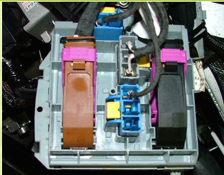
Place the connected front fuse box on its base, and connect the power bundle (see photo opposite).
